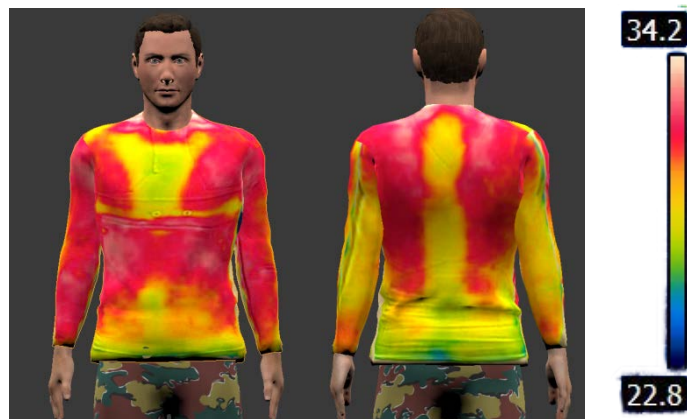
Fig. 3.2 Thermophysiological evaluation in DHM on the first prototype after 30 minutes of exposure
