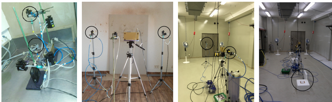
Fig. 3.2 Model rooms and instrumentation: small (1.5 m 3 ), medium (41 m 3 ), 2 × large (158 m 3 ). The circles indicate the sampling devices and, on the right photo, the deposition pads.
