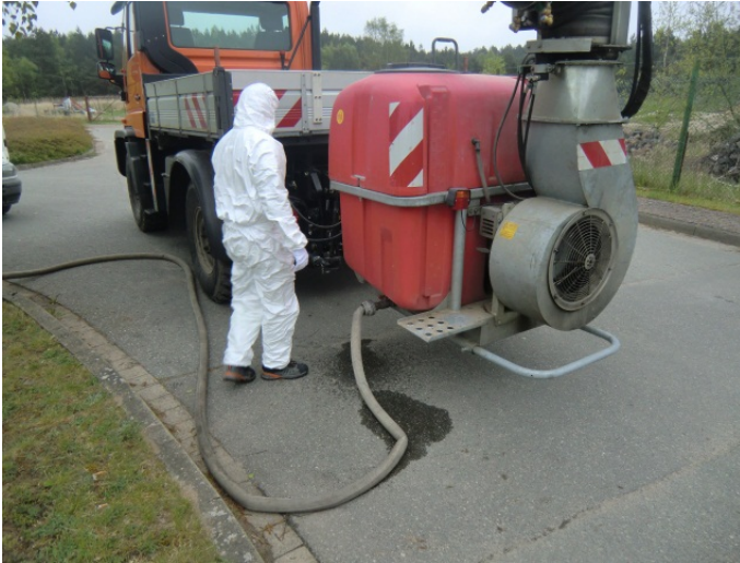
Fig. 3.8 Vehicle-mounted sprayer: Preparation of the Dimilin™ 80 WG suspension - Adding of water to the tank (company A).
