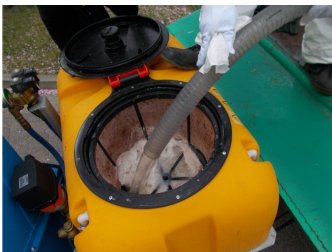
Fig. 3.13 Vehicle-mounted sprayer: Preparation of the Dimilin™ 80 WG suspension - Adding of water to the tank (company C). The strainer can easily be seen.
