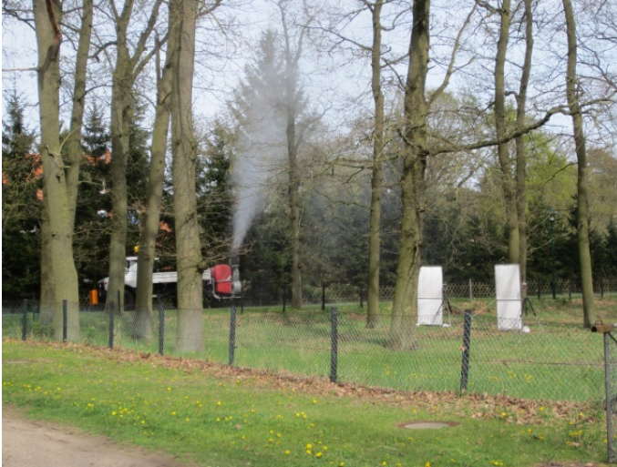
Fig. 3.28 Determination of bystanders` exposure during biocide application with vehicle-mounted sprayer. The picture shows the sampling VMS-application-dB-10 and VMS-application-iB-10 (company A).
