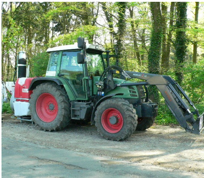
Fig. 3.4 Vehicle-mounted sprayer (tractor) (Dragone AZ with 800 L spray tank) of company B.
