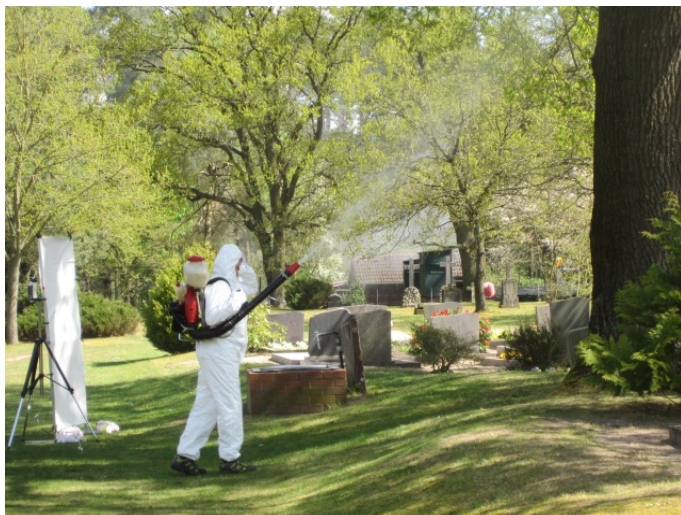
Fig. 3.30 Determination of bystander exposure during biocide application using a hand-held sprayer. The picture shows the sampling HHS-application-dB-11 and HHS-application-iB-11 (company A).
