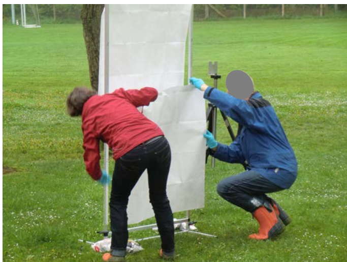
Fig. 3.27 Removal of a cut Tyvek™ sheet from the rack frame during the 2014 field study.
