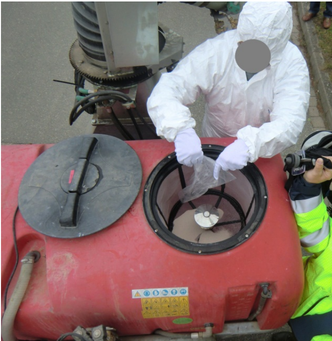
Fig. 3.9 Vehicle-mounted sprayer: Preparation of the Dimilin™ 80 WG suspension -Filling of the granules onto the strainer of the tank (company A).
