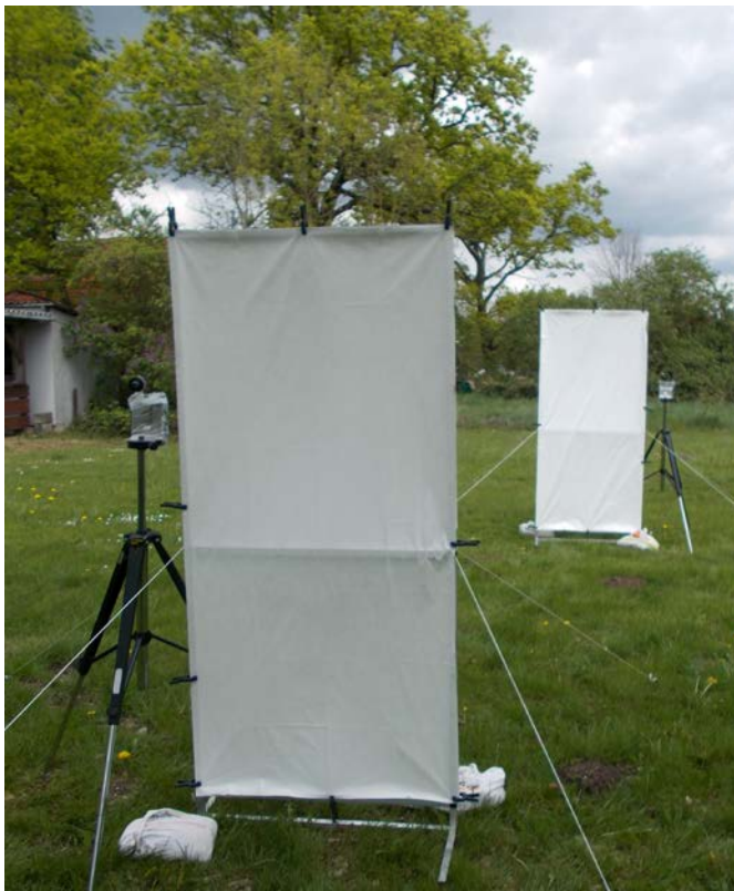
Fig. 3.26 Set-up to measure the dermal and inhalation exposure of bystanders during the 2015 field study.
