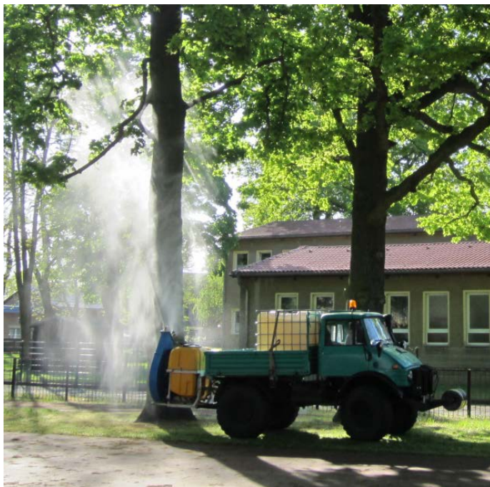
Fig. 3.5 Light truck with vehicle-mounted sprayer (Vicar Turbine 451 with 300 L spray tank) of company C.
