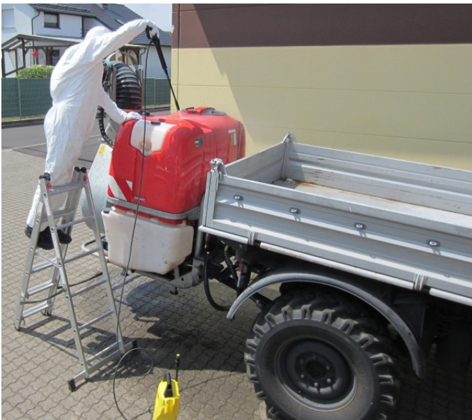
Fig. 3.19 Cleaning of a vehicle and a vehicle-mounted sprayer by a worker of company A (worker #8; 2015 field study). Standing on a ladder, the worker is cleaning the surfaces with a high-pressure cleaner.
