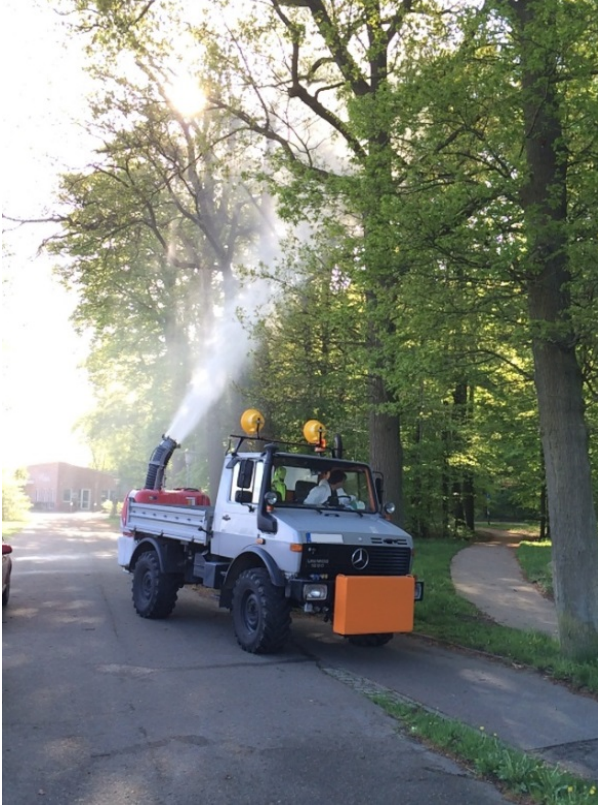
Fig. 3.1 Light truck with vehicle-mounted sprayer (Dragone AZ with 800 L spray tank) of company A.
