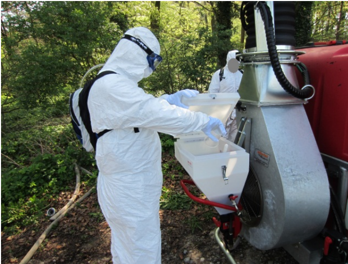
Fig. 3.11 Vehicle-mounted sprayer: Preparation of the Dimilin™ 80 WG suspension - Filling of the granules to the premix tank (company B).
