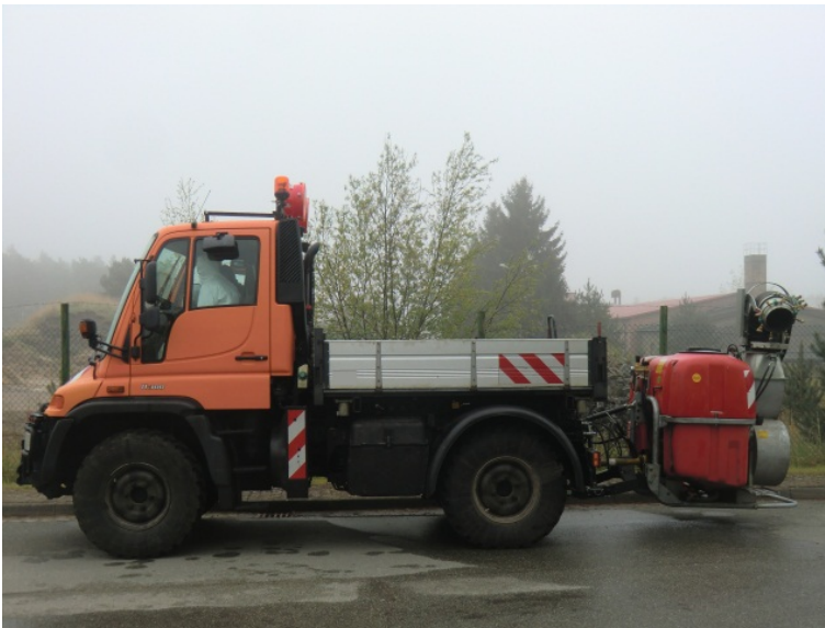
Fig. 3.2 Light truck with vehicle-mounted sprayer (Dragone AZ with 1000 L spray tank) of company A.
