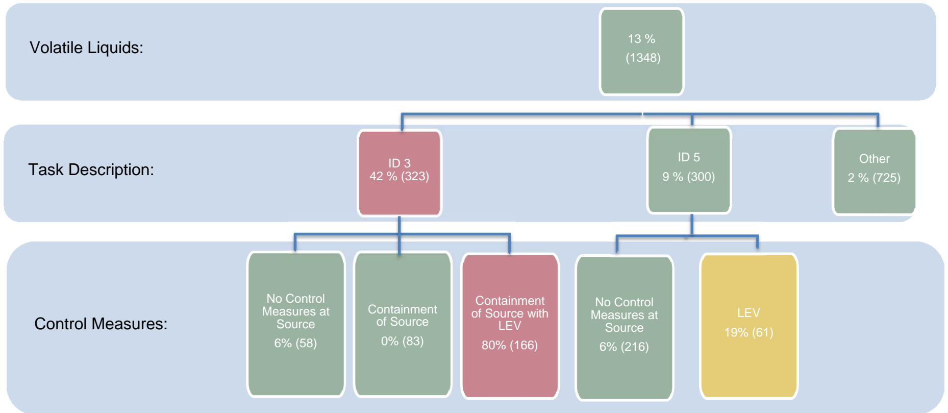
Figure 3.10 Tree describing the grouping of the various exposure measurements and codings by Stoffenmanager by the tools own parameters. Each element describes the total number of measurements within it (in brackets) and the percentage of non-conservative estimates. Task description 3 refers to “Handling of liquids where only small amounts may be released” and number 5 to “Handling of liquids using low pressure, low speed, or on medium sized surfaces”.
