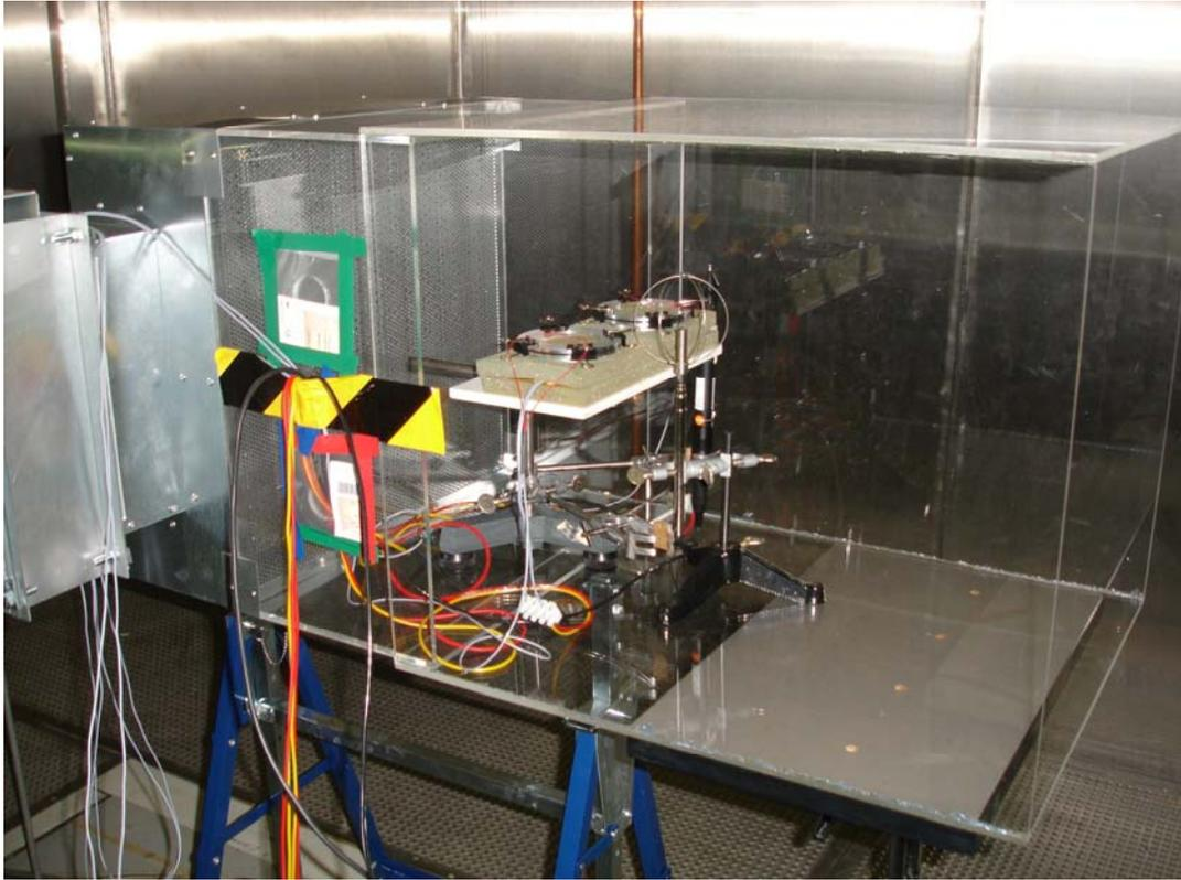
**Fig. 4.2** Tested specimen and the instrumentation for measurement of the evaporation rate and its dependence on the air parameters in the climate test chamber
