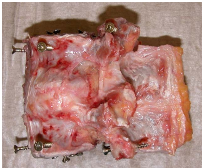
Fig. 2-3 Specimen 3012 L2-L3 with screws for improved fixation.
