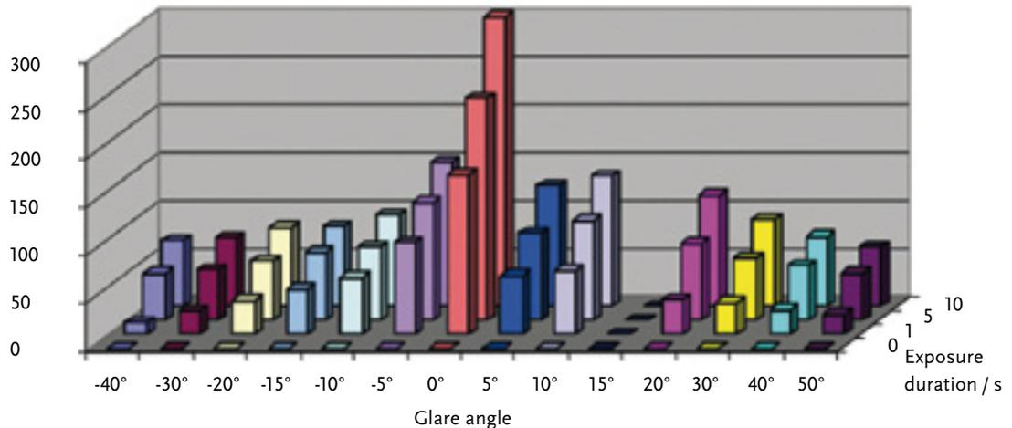
**Figure 11** Afterimage duration as a function of the glare angle and the exposure duration for a laser power of 30  $\mu$ W
