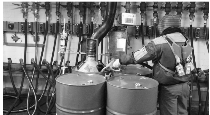
Figure 1. Different technical configurations for drum filling. Top left: according to existing control guidance sheet, top right: delivery tube surrounded by a trapezoidal extraction hood, bottom left: delivery pistol integrated into an extraction cup with exhaust ventilation, bottom right: manual filling pistol and external extraction hood (all photographs show sampling position 1 immediately at the LEV; additionally the photo at the bottom right shows the position 2 for personal air sampling).
