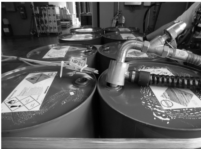
Figure 1. Different technical configurations for drum filling. Top left: according to existing control guidance sheet, top right: delivery tube surrounded by a trapezoidal extraction hood, bottom left: delivery pistol integrated into an extraction cup with exhaust ventilation, bottom right: manual filling pistol and external extraction hood (all photographs show sampling position 1 immediately at the LEV; additionally the photo at the bottom right shows the position 2 for personal air sampling).
