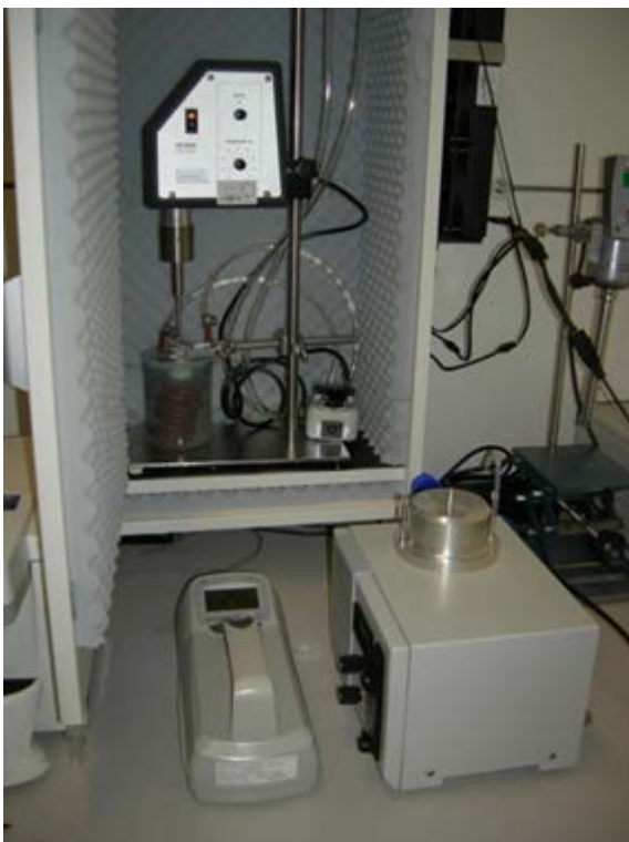
FIGURE 15: DISPERSION OF ZINC OXIDE WITH AN ULTRASONIC DISPERSER
