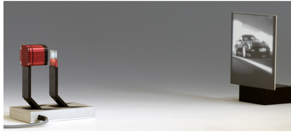
Test setup with collimated white LED for greyscale projection with QVGA resolution, projected flux 35lm
