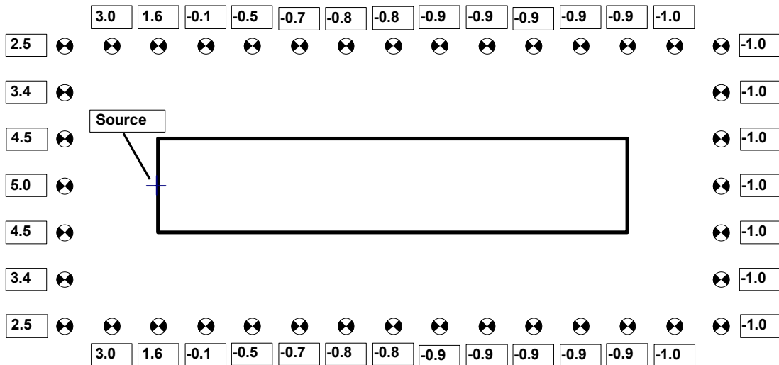
Fig. 5.7 Apparent directivity index DI' on a surrounding path at 1 m measuring distance in the room 10 m x 10 m x 6 m with mean degree of absorption 0.2
