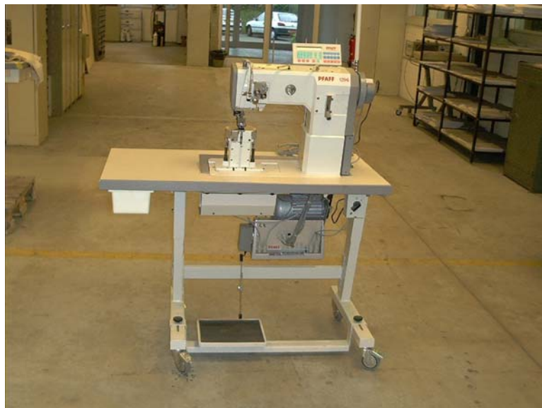
Fig. 7.4 Typical industrial sewing machine with concealed-body drive
