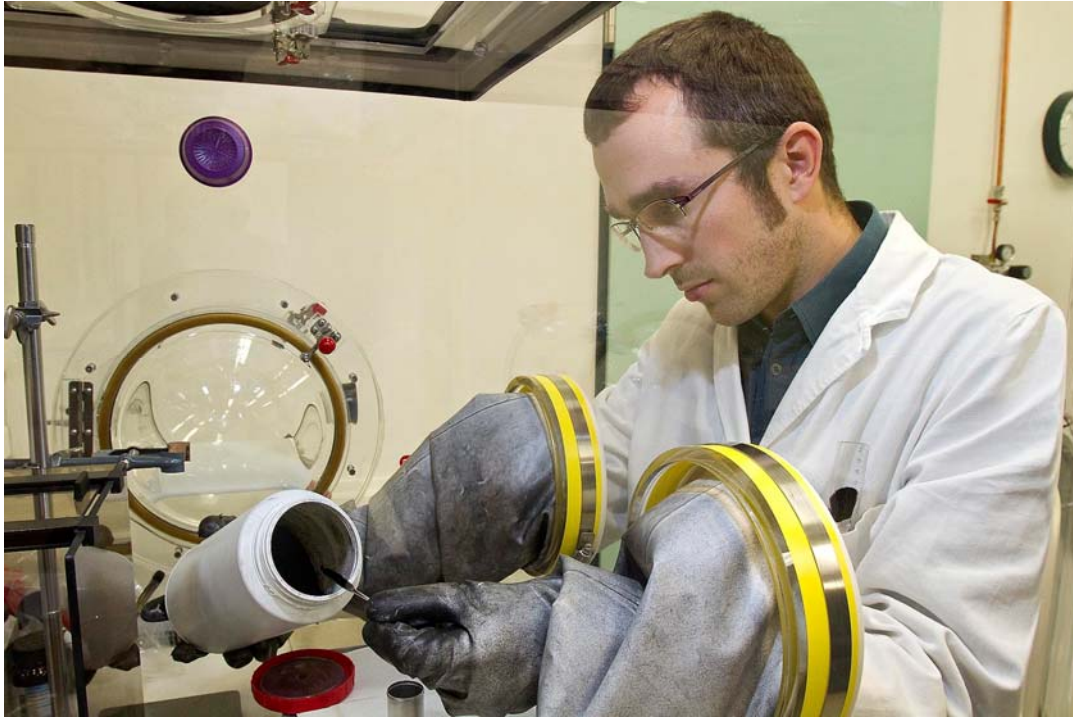
Figure 4: Handling nanomaterials in a glovebox as an example of an enclosed system at the workplace (photograph: BAuA/Völkner).
