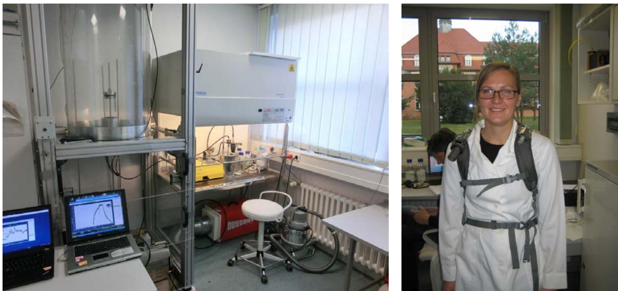
FIGURE 3: TEST BENCH FOR RELEASE EXPERIMENTS WITH MWCNT (LEFT) AND PERSONAL SAMPLING WITH A PORTABLE DEVICE (RIGHT).
