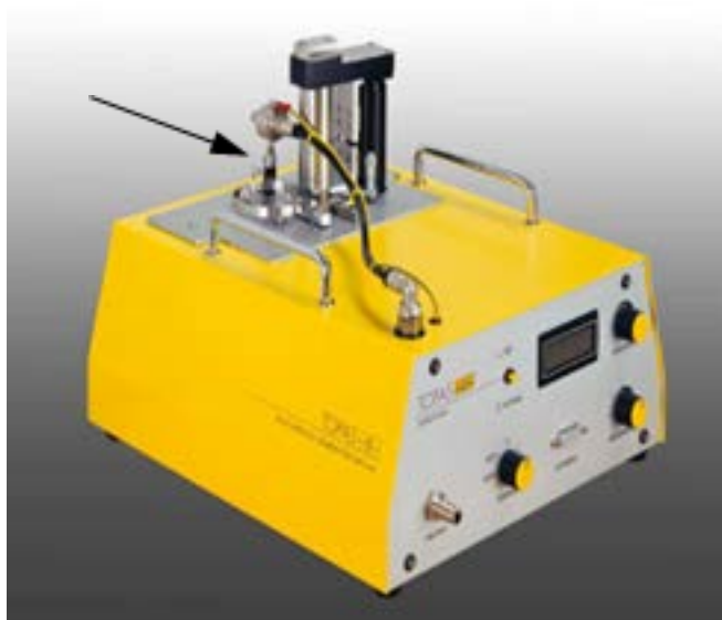
FIGURE 3: DUST GENERATOR SAG 410/U 1 FROM TOPAS1 (TOPAS GMBH 2009), ARROW: NOZZLE
