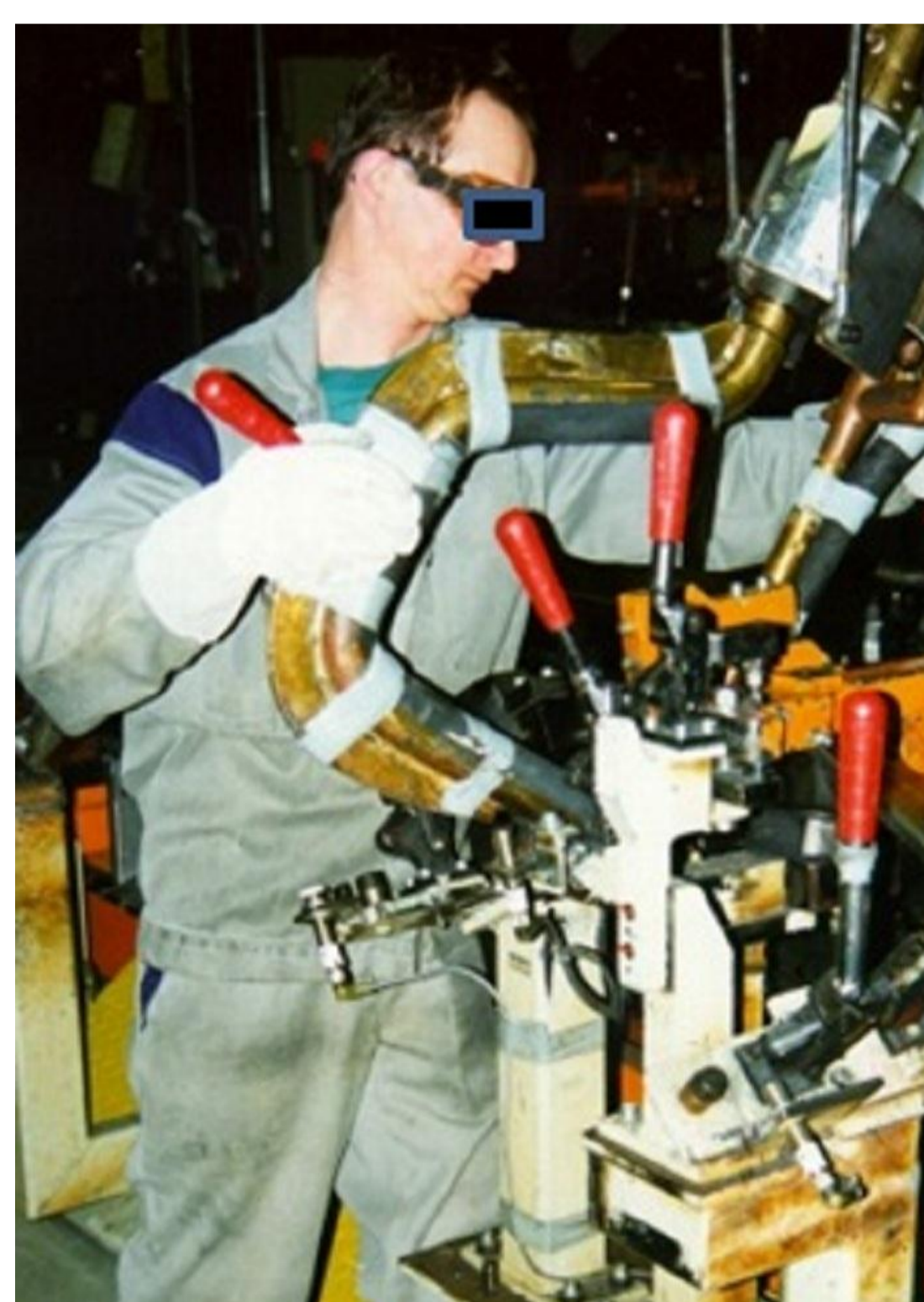
Figure 1. Worker with resistance welding gun
