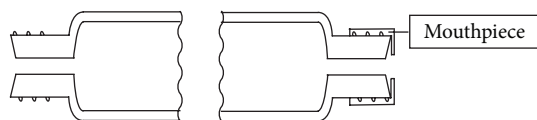
FIGURE 2: Sketch of the valveless gas sampling tube, ready for sampling; open-top cap screwed on as a mouthpiece.
