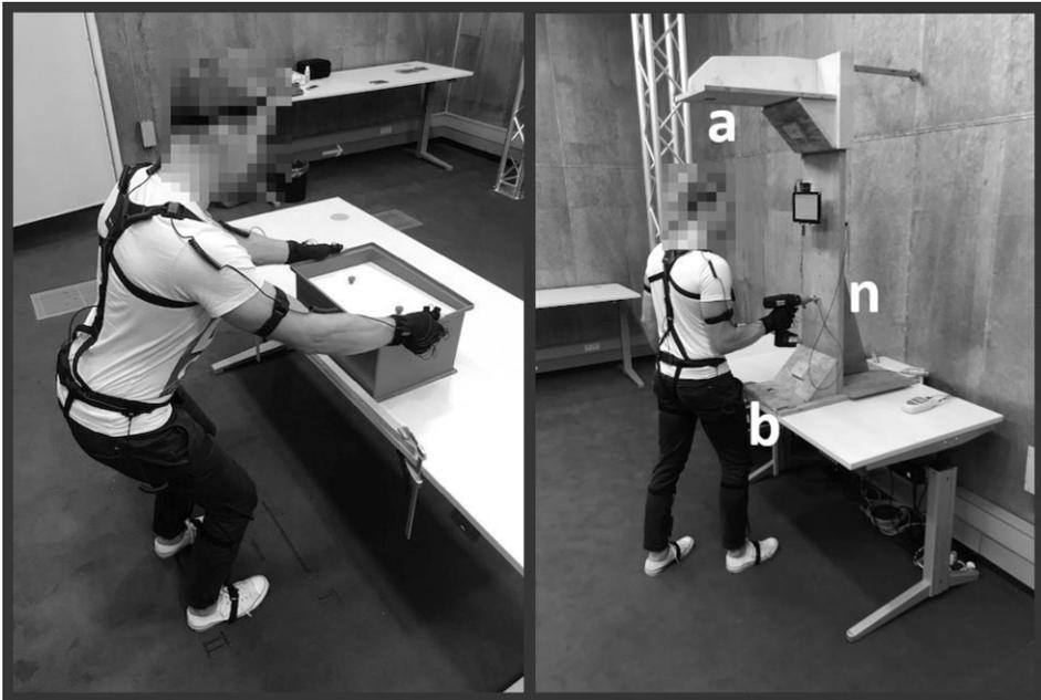
**Figure 1.** MMH task and assembly activity with a drilling machine in neutral posture.
