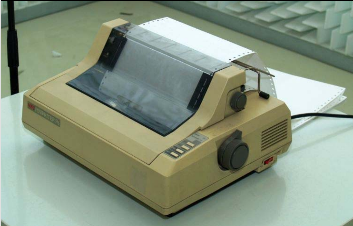
Abb. 5.3 Nadeldrucker (Kategorie C.3 - Character- and line-printer)
